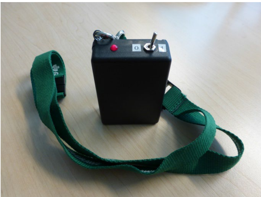
Abb. 19 Acoustic and optical 10 s clock (developer: Ing. Heinz Gressenberger, A15)
