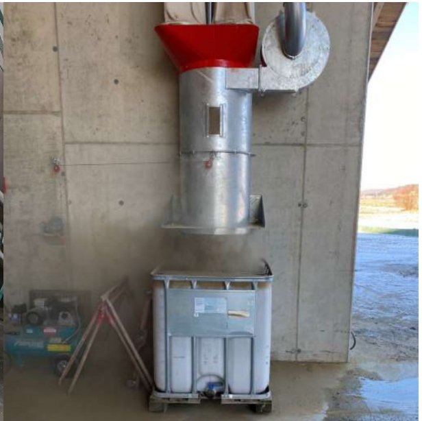
Abb. 8 Dust removal system for bedding
